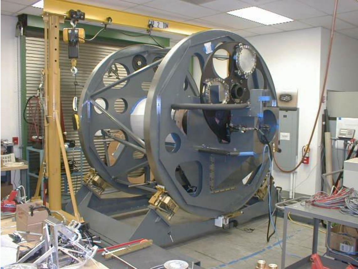
Figure 2. A recent image of IMACS partially assembled. The carriage, roller assemblies, DSS wheel, structure, and testing drive assembly can be seen.
