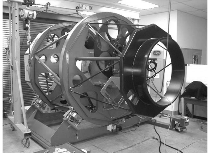
FIG. 21.—An early stage of assembly of IMACS in the Carnegie Observatories shops. This photo shows the carriage, with its self-steering rollers supporting the rotation of the IMACS structure assembly. The rotating assembly consists of two monocoque disks connected by the main truss, the secondary truss ( black ) supporting the cantilevered rotating portion of the utility wrap, and the MOSS. Also visible in the photo is the primary structure ( wheel ) of the disperser server that carries the spectrograph dispersers and accessories.
