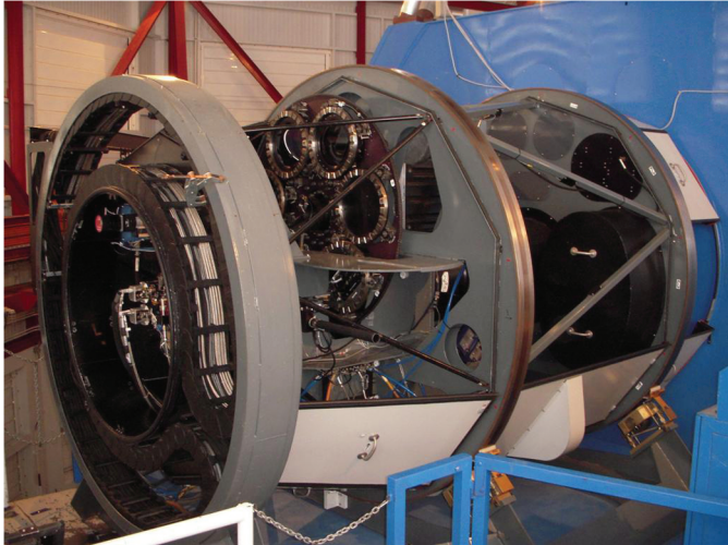
FIG. 20.—IMACS installed at the west Nasmyth platform of Baade, with most of the enclosure panels removed. This photo shows the carriage with its self-steering rollers supporting the rotation of the IMACS structure assembly. The rotating assembly consists of three sections. (1) Main structure—two monocoque disks (FOSS and MOSS) connected by the gray square-tube main truss. This section encloses the collimator and its baffle and the f/4 train: filter server, shutter, f/4 camera, and Mosaic-1 CCD camera (all far side, not visible). (2) Forward compartment, the short projection from the FOSS disk to the Nasmyth instrument rotator. This section encloses the field lens, the mask server, the three guiders, and the calibration unit. (3) Aft compartment—the secondary truss ( black bars ) supports the cantilevered, rotating portion of the utility wrap at the back of the instrument. In this section is the MOSS box, the weldment to which the collimator and f/2 and f/4 cameras are attached—in other words, the spectrograph. Also visible is the primary structure ( wheel ) of the disperser server; the gratings and grisms face forward and are identifiable by the index rings used to latch a selected unit to the spectrograph. Also enclosed in the aft compartment are the f/2 train: filter server, shutter, f/2 camera, and detector. The filter server and detector are slightly visible within the utility wrap.
