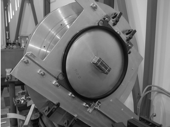
FIG. 25.—Mask server, early in the design development phase. The mask assembly consists of a C-channel hoop that holds the mask and two opposing wings that attach to the hoop. The beveled straight edge on each wing engages with the V-roller wheels to guide the mask assembly between the mask cassette and the in-beam position. In the lower half of the image, the air-cylinder insertion actuator and linear bearing guide are visible. This picture shows the testing of the mechanism under varying gravity orientations, using a gap bed lathe in the Carnegie shop to rotate the unit (this test was done prior to the assembly of the main structure and carriage). The large weight at the center of the mask simulated the estimated mass and center of gravity of the Durham IFU, which was much heavier than a single multislit-mask assembly.
