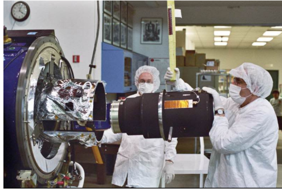
Fig. 10.— A.M. and S.E.P shown inserting (via a crane/strap) the CM into the mylar-covered 200K shield within vessel section 1. The load ring is the gray ring at its end. The copper-colored rectangular patch on the body of the module is one of the three Minco heaters.
