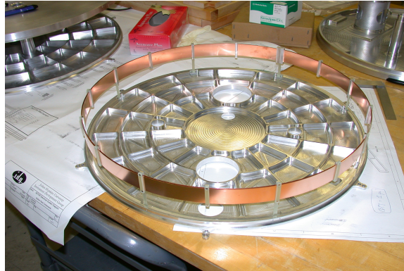
Fig. 13.— The copper capacitor under construction and mounted on the aluminum back plate of the shield dewar before welding. The milled pockets in the back plate are for lightweighting.
