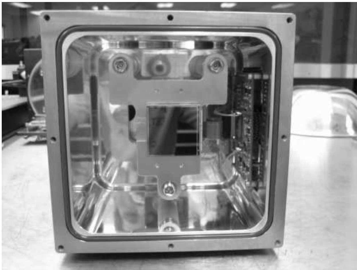
Fig. 1.— The Teledyne Hawaii-2RG array can be seen mounted in the center of CAPSCam-N, shown here with the Barr Associates filter/window removed. The Hawaii-2RG array is approximately 2" by 2" in size.
