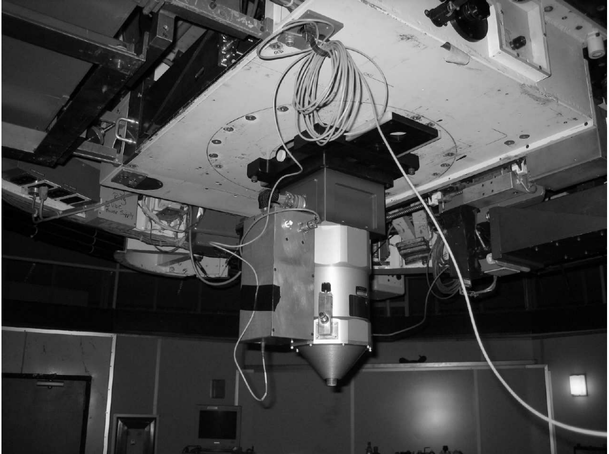
Fig. 2.— CAPSCam-S is shown mounted at the Cassegrain focus of the 2.5-m du Pont telescope at Carnegie's Las Campanas Observatory in Chile.
